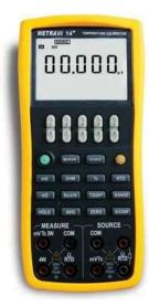
Provides DC Voltage, DC current, simulation transmitter, Frequency & Pulse outputs
