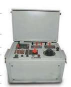
It is suitable for testing distance relays.
