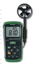
Displays Air Velocity and Temperature together
