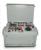
Current output is continuously variable and the output is taken out through a multi range C.T. The secondary is connected to an ammeter scaled in 0 to 100%
