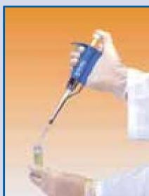
1. Fill the pre-dosed vial with the sample
